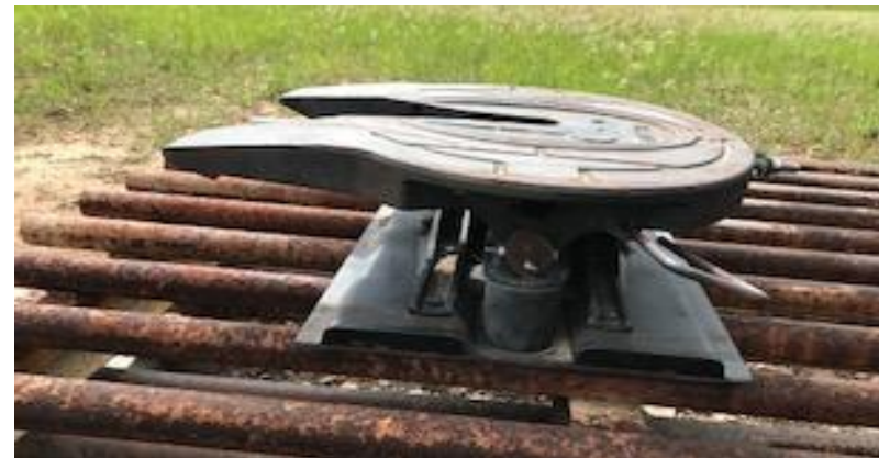
Holland FW 1560-C 5 th Wheel Plate, fully oscillating, heavy duty, Perfect for low profile trailers, saves wear & tear on truck suspension And frame, unused. $1200.00
